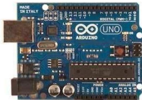
Gambar 2.3 Arduino Board
